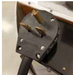
Receptacle / Plug Config. & NEMO no. 6-30
